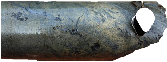
Figure 4: Massive sulphide mineralization in hole IB18-009 at 79.57m to 80.02m downhole – Sphalerite (yellow, grading 40.9% Zn) is the dominant mineral present.
