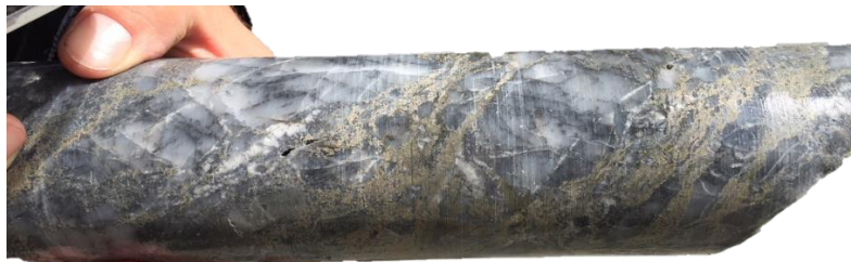
Figure 5: Fracture fill sphalerite (zinc sulphide) in silicified sedimentary breccia from hole IB18-008.
