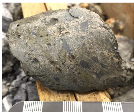
Figure 3: Massive sulphide mineralization - Hole IB18-003 (low core recovery). Shale and pyrite clasts in sphalerite (zinc) rich matrix.
