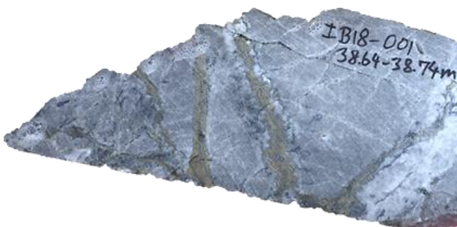
Figure 4: Sphalerite (zinc), galena and pyrite in fracture fills in carbonate - typical mineralization seen in Holes IB18-001 and IB18-002 (HQ Core).
