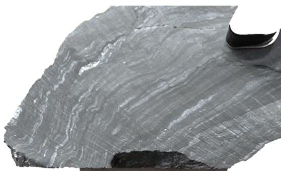
Figure 2: Finely laminated pyrite-sericite schist.
