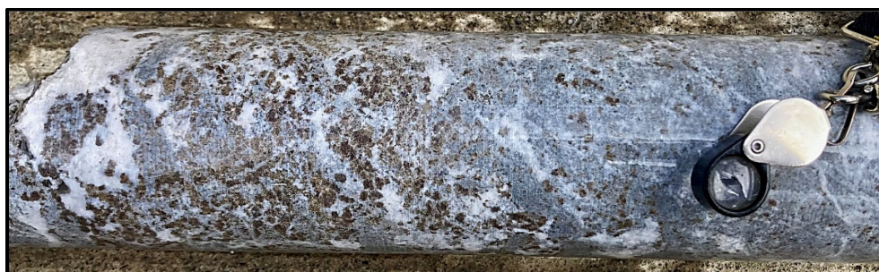
Figure 2: Drill Hole IB26-051 – Coarse Crystalline Sphalerite (Zinc)
